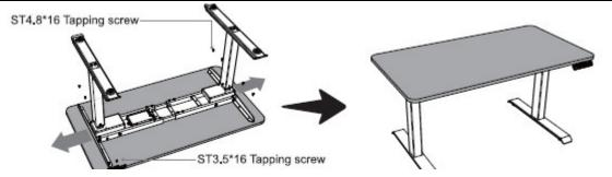
The frame width is adjustable: 40 inch~ 60 inch, which is suitable for different desktop
